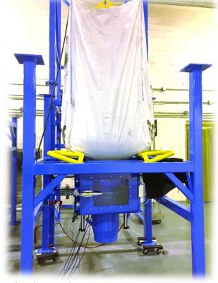
Lower Section installed atop mixer. Contain-It™ Chamber with Massage-It™ bag agitation system shown.
