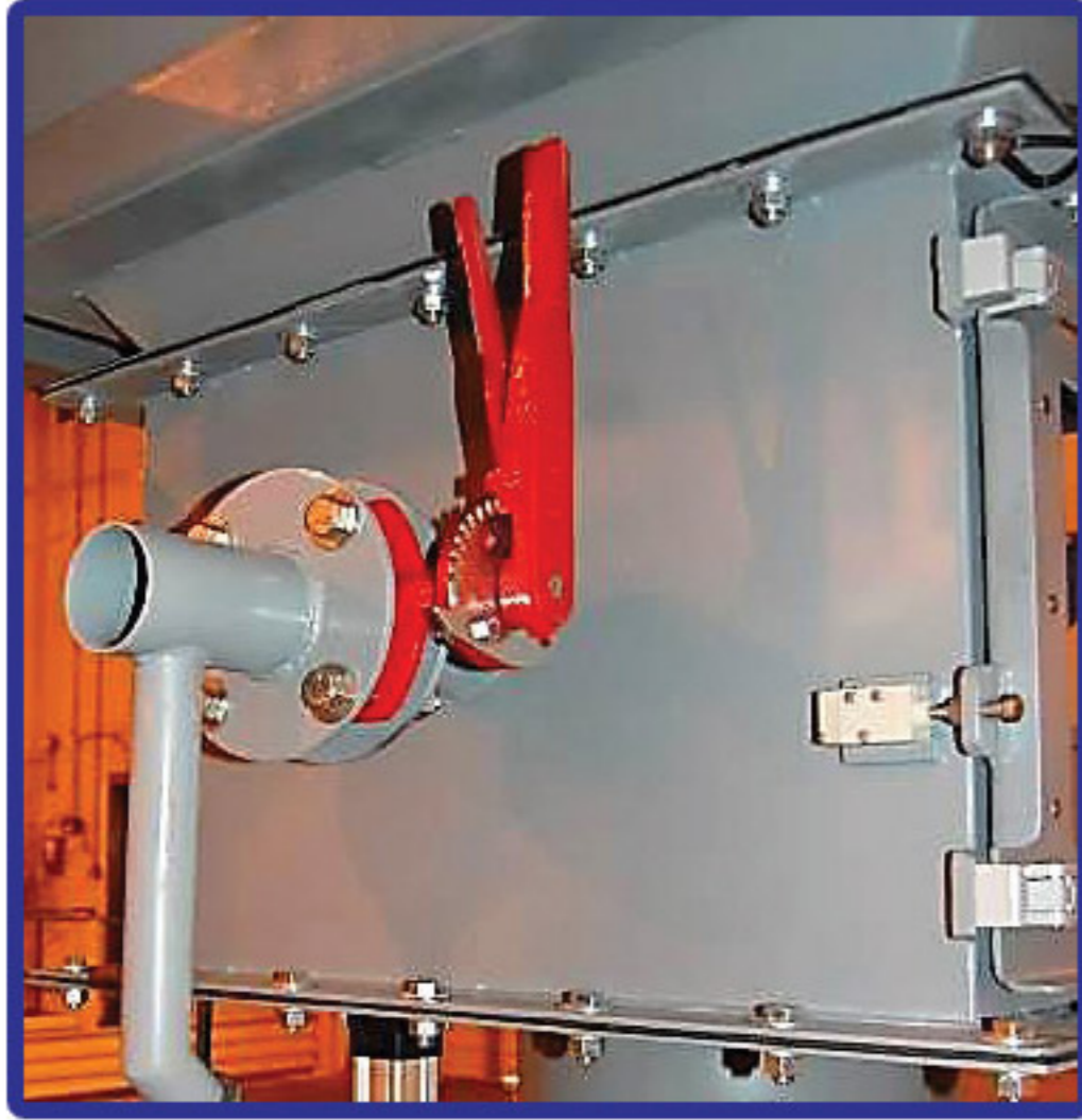
Dust Collection - 350 CFM for proper Dust Collection on Contain-It™ chamber
