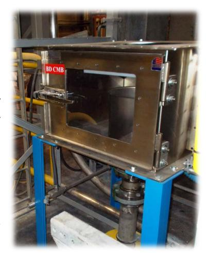
The Close-It™ can actuate only when the door is closed, thereby protecting operators.
